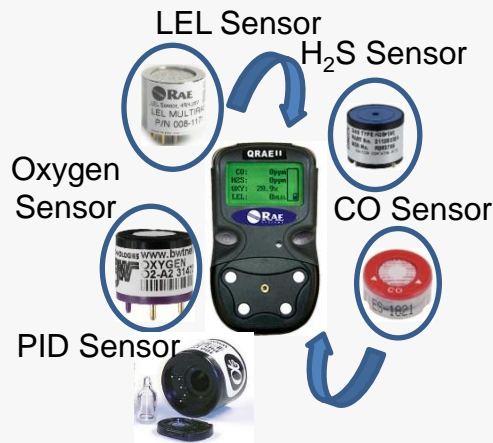
A Typical 4-Gas Handheld Detector Construction (RAE Systems)
